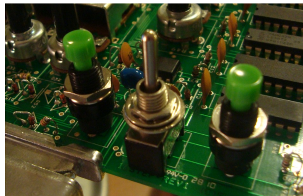
Hold and step switches
