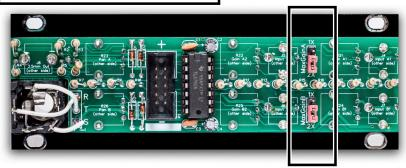
Jumper Select 1x or 2x Gain Per Channel
