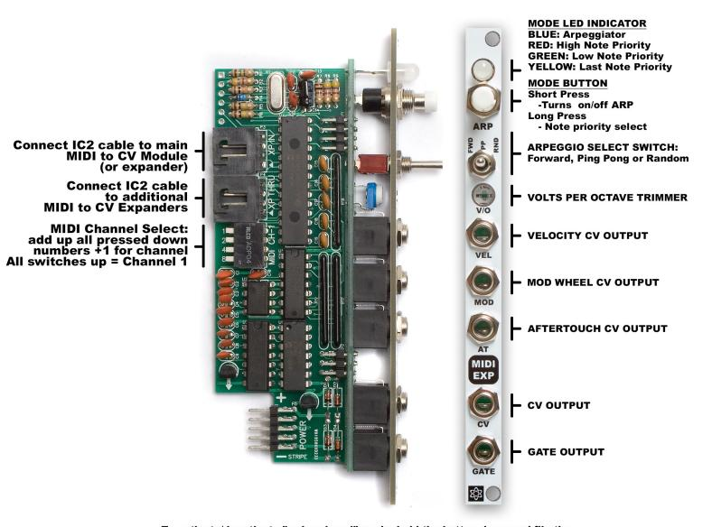
To activate/deactivate "order played" mode, hold the button down and flip the switch to any new position within 2 seconds. The LED will light green when "order played" mode is activated or red when deactivated.
